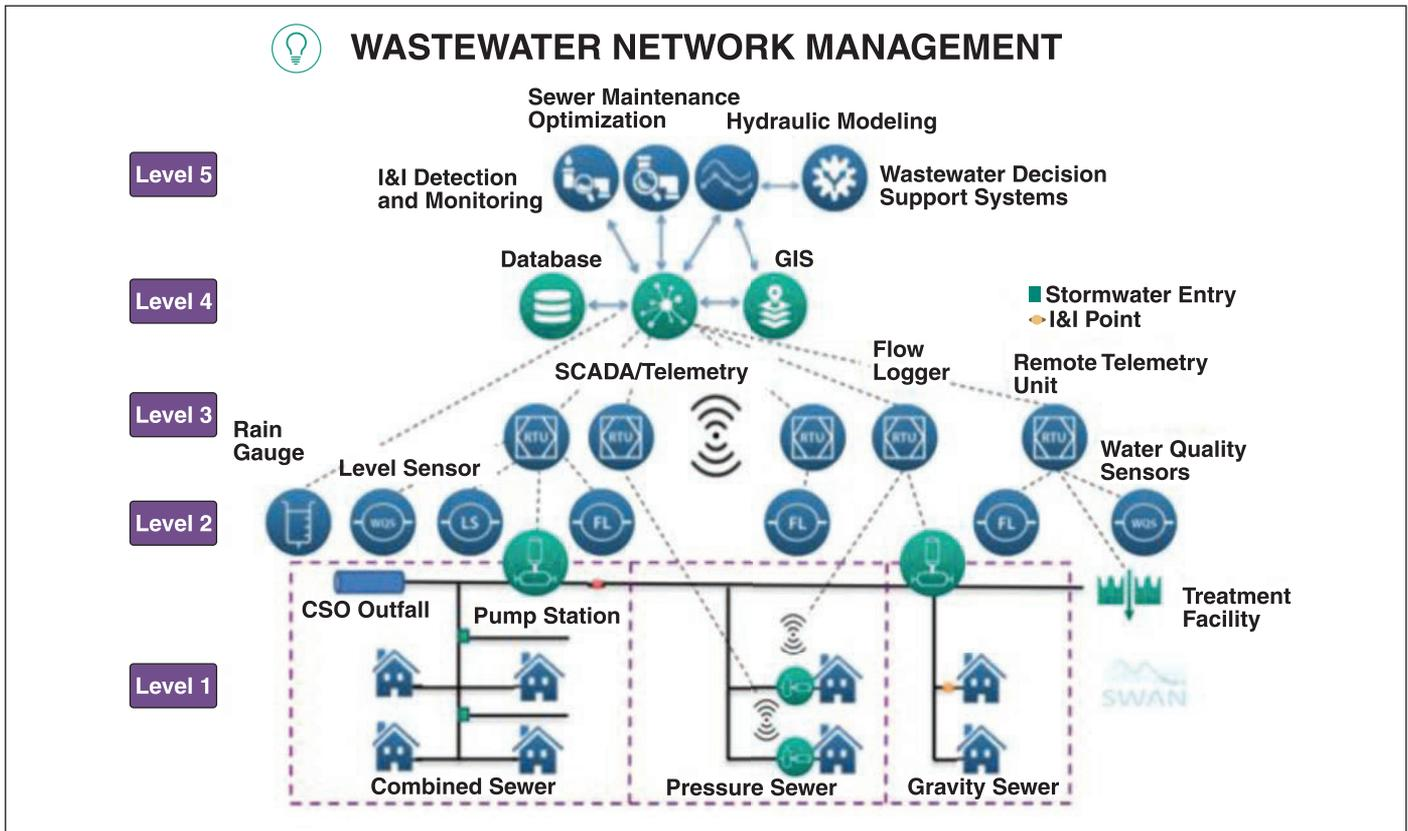
Figure 5: SWAN Wastewater Network Management Solution
