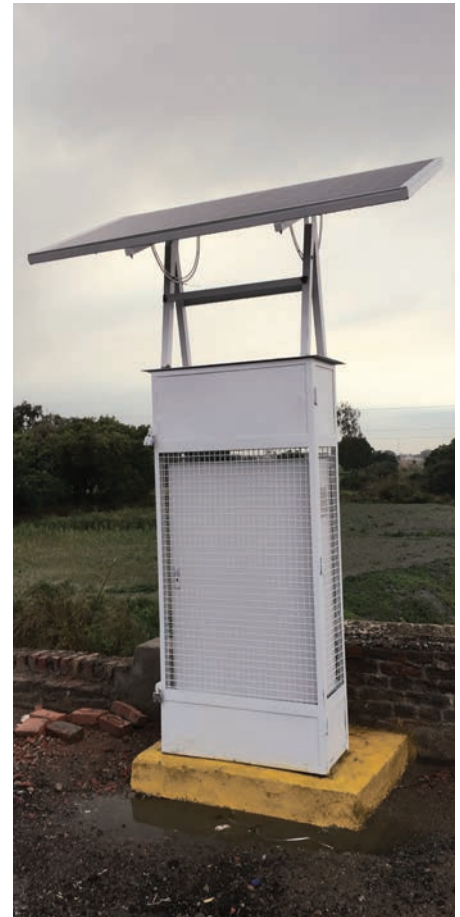
s::can Energy Autarkic – s::can Monitoring Station
