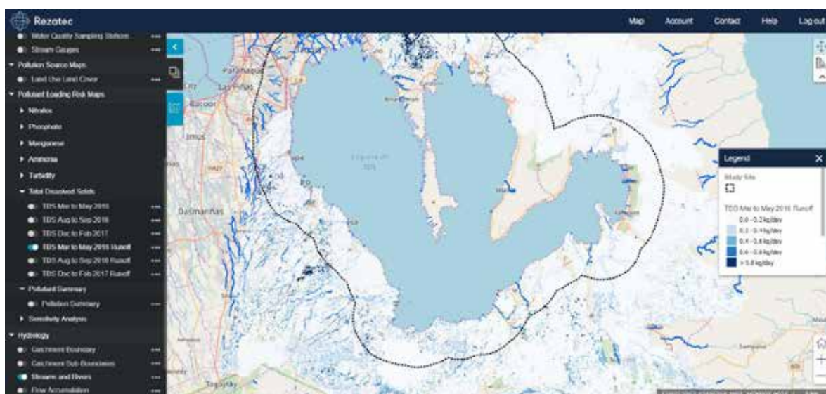
Figure 2: Illustrative example of data visualisation afforded by satellite imagery combined with the hydrological model of Laguna de Bay. The image reveals an analysis of the average volume of Total Dissolved Solids (TDS) as run-off during a 3-month period.
